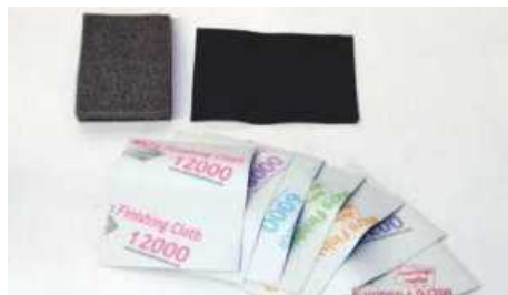
▲ Likewise, the cloths are printed with grits as well as a different colour for each
